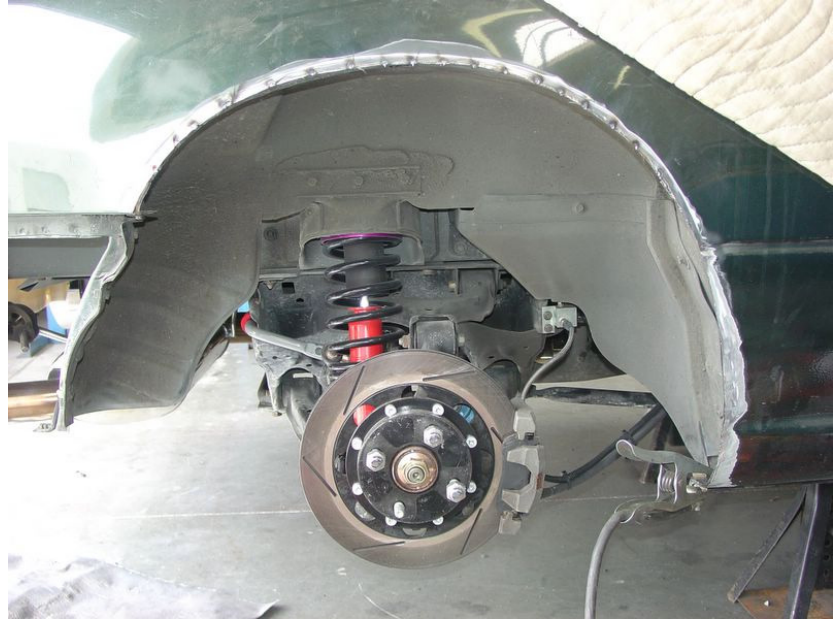
Fully tack welded fender section ready for final welding and grinding.
