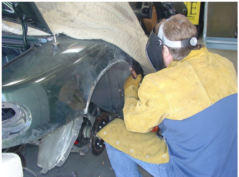
Jeff starts to finish off the sections of weld between the tacks. Again, take your time and allow the fender to cool between welds. Switch from front to back and side to side to help stop deformation on the panels.
