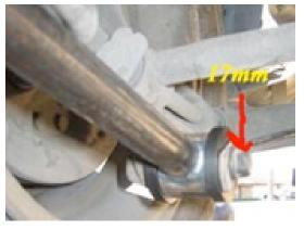
**Step 3:** Remove 17mm bolt from the stock trailing links where it bolts to the wheel hub.
