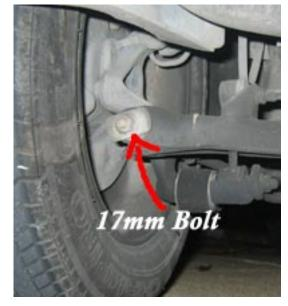
**Step 5:** Install new black sway bar bushing relocation brackets using the stock nut and bolt to affix them to the lateral cross-member. Be careful not to cross thread either the nut or bolt when tightening them down.
