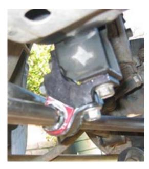
**Step 9:** Attach end links using supplied hardware.
