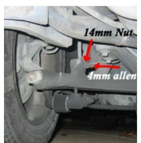
**Step 2:** Unbolt both passenger side and drivers side end links from the lateral link. [Use 4mm Allen head wrench and 14mm closed end wrench]
