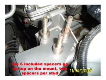
22. Replace the three 15mm mounting nuts on the studs and tighten all mounting bolts and nuts down. Start with the frame rail mounting bolts, then the fender well nut, then the engine stud nuts.
