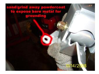
19. Insert the ¼" bolt into the small hole on the tongue extension with the head of the bolt facing downward. With a flat washer on both sides. Tighten down with respective nut.
