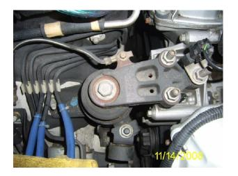
8. Remove one 8mm bolt from mount arm to release ground wire.
