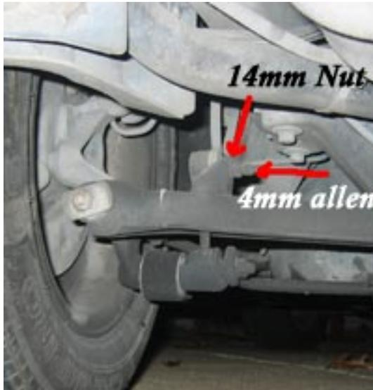
**Step 2:** Unbolt both passenger side and drivers side end links from the lateral link. [Use 4mm Allen head wrench and 14mm closed end wrench]
