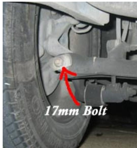
**Step 5:** Install new black sway bar bushing relocation brackets using the stock nut and bolt to affix them to the lateral cross-member. Be careful not to cross thread either the nut or bolt when tightening them down.
