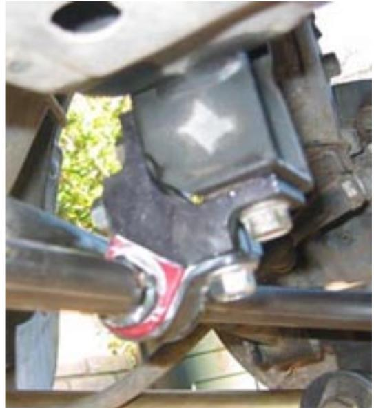
**Step 9:** Attach end links using supplied hardware.
